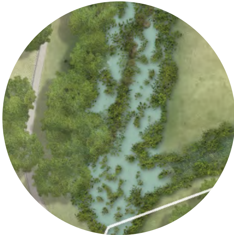
Detail plan showing the central Army Camp Basin area with sediment pond, ephemeral wetlands and native tree planting.
